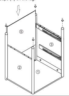
8 Add piece 4 to the unit using wooden dowels (F), Screw (G).
